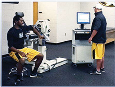
For IR/ER 90 Abduction pattern, Long has the athlete sit on a stool to the side of the dynamometer.
