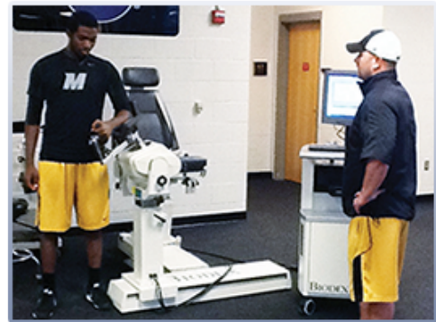
For IR/ER in modified neutral, Long has the athlete stand to the side of the dynamometer.
