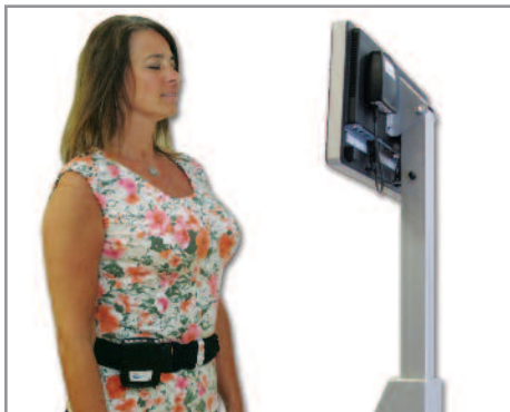
Vibrotactile cueing allows patients to get positional feedback with their eyes closed.
